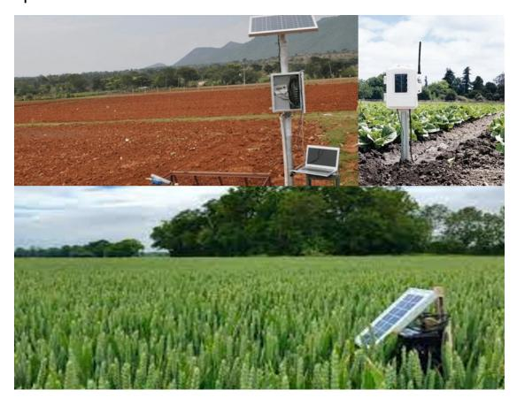
Sensors are mechanisms of automatic sampling and rapid measurement. There are several categories of sensors such as crop sensors, field sensors, soil sensors, plant sensors, weed or infestation sensors. The special sensors are placed in the fields and collect information on temperature, humidity, weather conditions, diseases, etc. By using such sensors, each farmer can have direct access to a range of field-critical information related to normal growth and crop needs.
