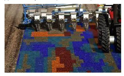
Variable application systems are agricultural engineering systems that are installed on agricultural machinery and change the amount of application of inputs (water, seed, fertilizers, pesticides, etc.). Also they are able to change the type of inputs (seed variety, fertilizer type) the same time as they apply the inputs, according to the needs of each point of the field. This technology is based on mapping techniques or sensors.
