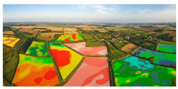
Yield monitoring systems are systems for measuring and recording the yield of a crop at harvest point. The data obtained, in combination with the global positioning system (GPS) and the geographic information systems (GIS), are giving important information about the
